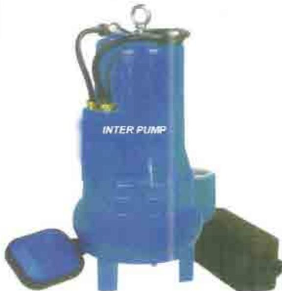
WQ series submersible sewage pump is mainly comprised of three parts: pump, mechanical seals and motor. Pump is at the lower of sewage pump, and the structure is impeller and shell. Motor located at the upper part of the motor pump, which is the single phase or three-phase electric motor. Mechanical seals are between pump and motor and it is a kind of double and mechanical seals, "O" rings are applied in all static joints of the submersible pump.
